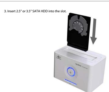
3-1. When the eject button is upright, the NexStar Hard Drive Dock is ready for use.
